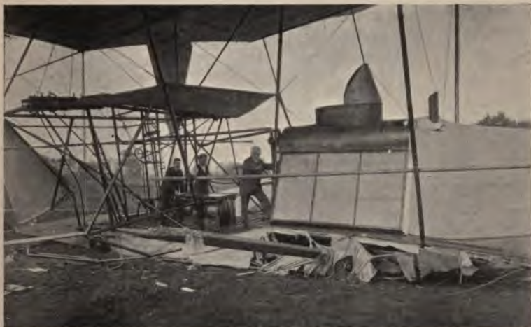
Fig. 82.—The condition of the machine after the accident. One of the broken planks that formed the upper track is shown. It will be observed that the wheels have sunk directly into the ground without leaving any tracks, showing that the machine did not run along the ground, but came directly down when it stopped.
